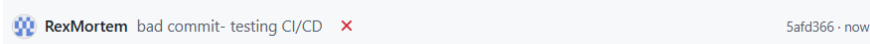
Figure 11: A failing commit on the main branch as it appears on GitHub. The test.yml workflow has run cargo test against the new commit, the unit tests have failed, and the failure is reported directly against the commit; this prevents broken code from being silently deployed.
